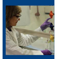
The fume hood is often the primary control device for protecting laboratory workers when working with flammable and/or toxic chemicals.
