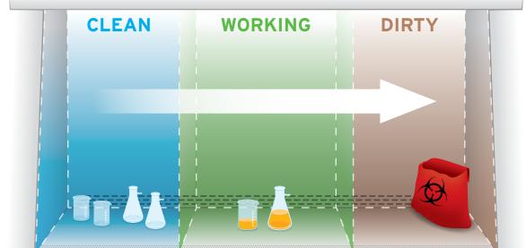
Distribute items evenly in the work area to help maintain uniform airflow. Supplies and equipment (especially aerosol generators such as vortex mixers or tabletop centrifuges) should be as close as practical to the rear of the work area, away from the front grill.
