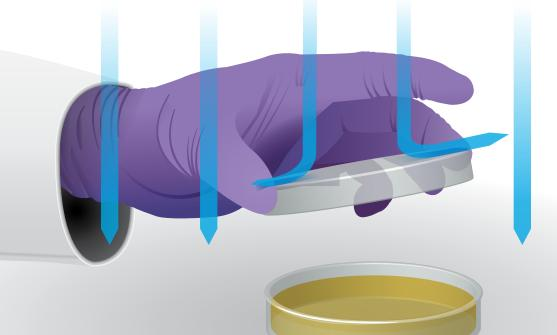
When working with petri dishes and tissue culture plates, hold the lid above the open sterile surface in order to minimize the impaction of air downflow.
