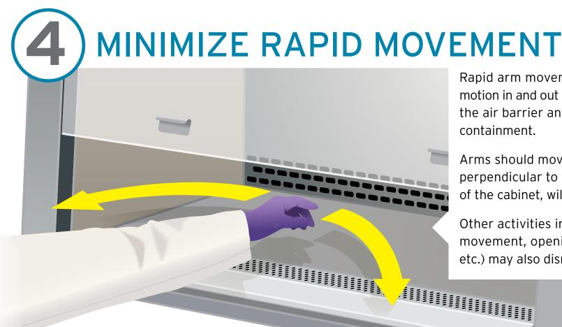
Rapid arm movement in a sweeping motion in and out of a BSC can disrupt the air barrier and may compromise containment.
