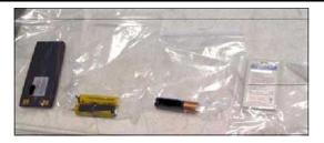
Place the same type of batteries together and then place clear tape over the tops
